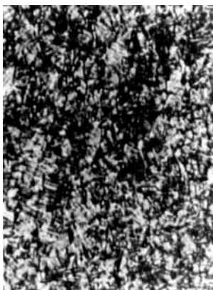
FIGURE 7 Optical textures observed from \text{PcH}_2 ( 1c : \text{Pc}-\text{OC}_{12}\text{H}_{25} ) at 250^\circ\text{C} and \text{CuPc} ( 2c ) at 220^\circ\text{C} ( \times 300 ).
